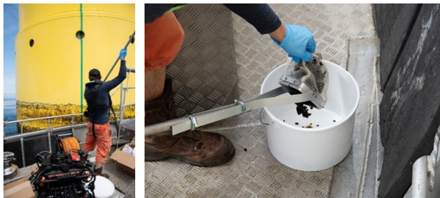
Figure 3.2. Scraping samples at a turbine tower. Photo Karsten Dahl.
