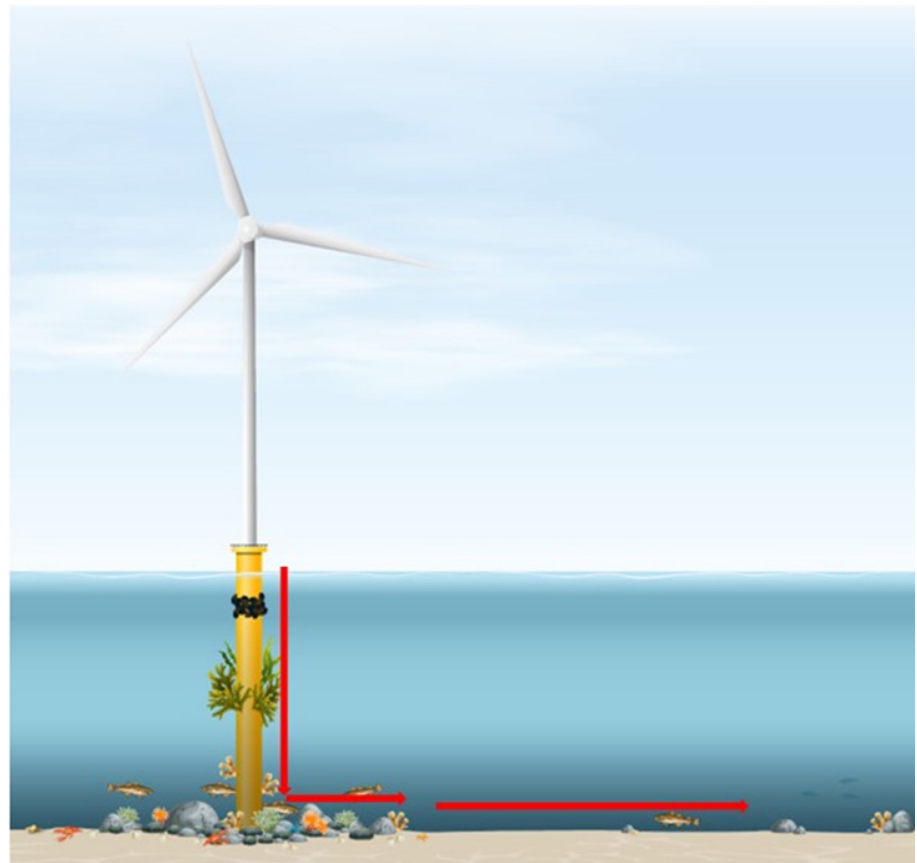
Figure 3.4. Overview of the wind turbine and ROV survey transects. The figure illustrates the layout of the wind farm, including the scour protection and the transect investigated by the ROV.
