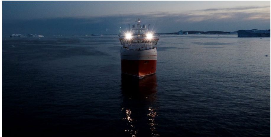
Figure 3.4. The main floodlight onboard R/V TARAJOQ used to detect icebergs or other navigational risks during sailing in ice-infested waters. Photo: Alex Rivest.
