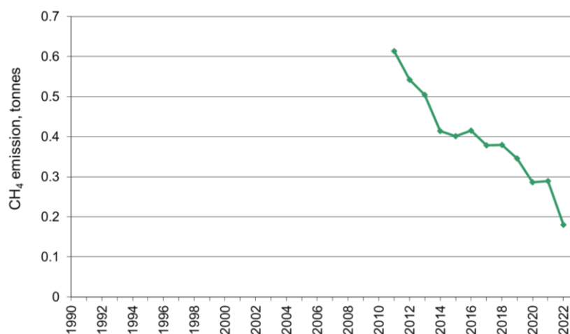
Figure 3.5.27 CH 4 emissions from flaring in gas transmission and distribution.
