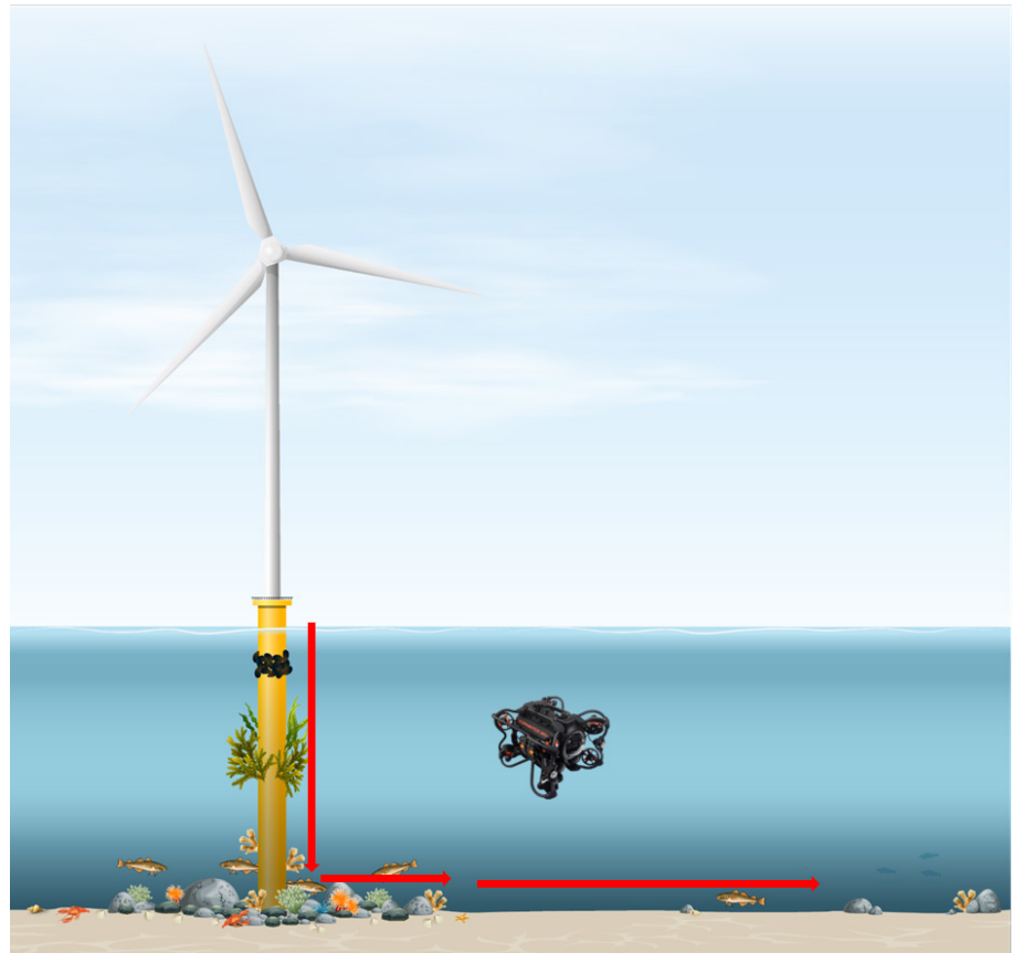
Figure 3.5. ROV investigation of the monopile, the seabed close to the monopile and in the vicinity of the monopile.
