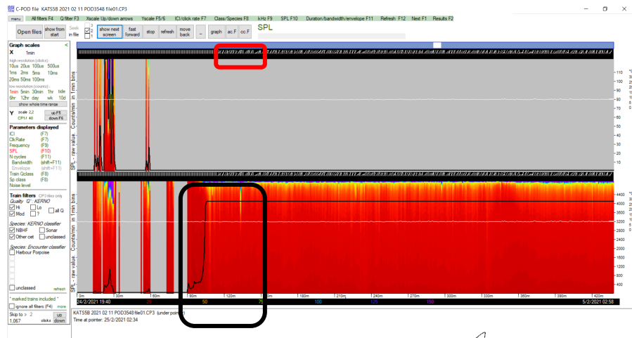
Figure 3.2. Example of a CPOD that has been trawled. Deployment KAYD 2B. Notice how the background noise increases and saturates (red colour in lower graph inside the black rectangle) along with a change in angle (red rectangle in upper graph).
