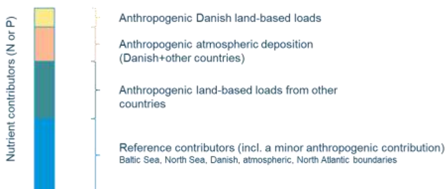
Figure 2-1 Schematic figure showing the contributors to the concentrations of nutrients in a specific water body. The relative parts of the different contributors will vary significantly between the different water bodies.
