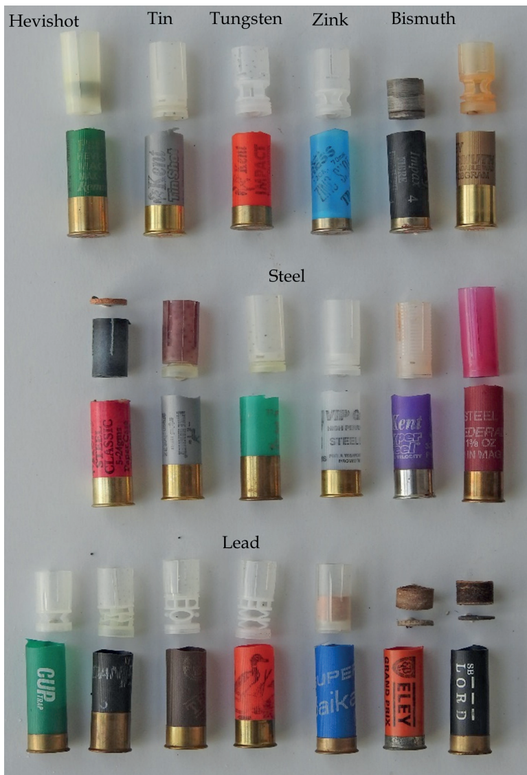
Figure 5.17. Wad construction in a selection of shotgun cartridges. All caliber 12. Bottom: lead; Middle: steel; Top (from left): hevishot, tin, tungsten, zink and two bismuth. See text for details.
