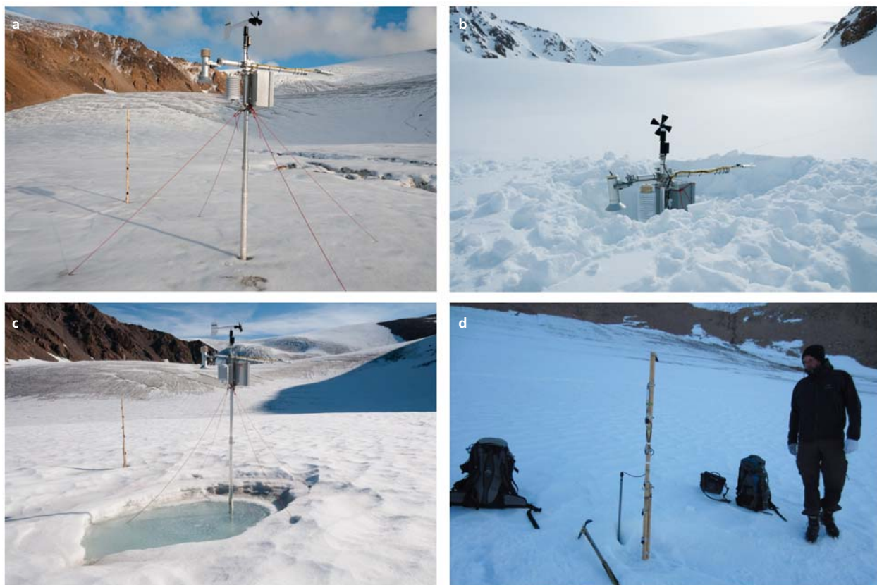
Figure 6.4 The AWS on Freya Glacier after a) the installation in August 2011. b) buried in snow in April 2012 and c) in August 2012. The refrozen melt water pond around the AWS in August 2012 illustrates the problem of a thermal impact of the measurements. d) Snow and icelfirn temperature measurements in the accumulation area. Photo: Gernot Weyss.
