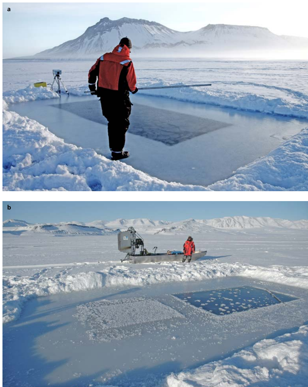
Figure 6.32 Opening cut for a) the in situ frost flower growing experiment and b) the frost flowers formed on new ice overnight. Photo: Jakob Sievers (top) and Søren Rysgaard (bottom).
